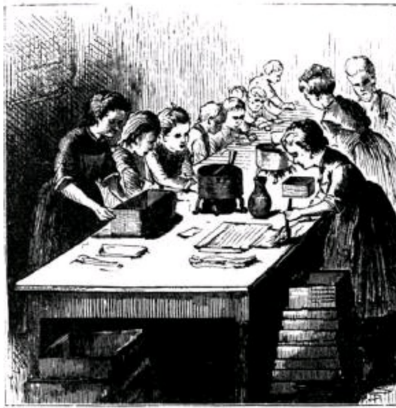
Hand-gluing paper bags and boxes. A machine to mass-produce flat-bottom grocery bags was patented in 1883.
