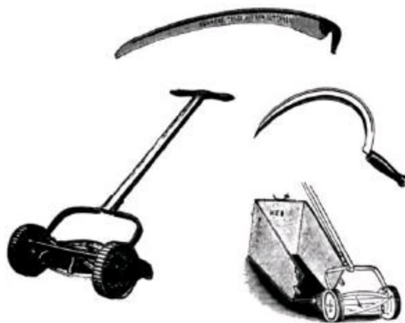
(Clockwise) Scythe cutting blade; hand-held grass sickle; rotary blade mower and grass catcher; mower after Budding's 1830s' model.
