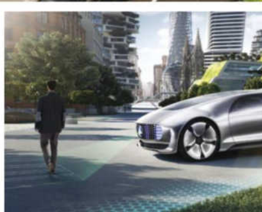
Mercedes-Benz's F 015 concept has laser projectors and LED screens for other road users and pedestrians
