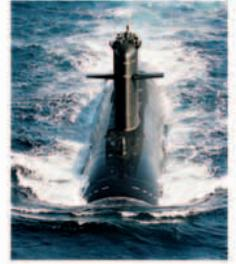
**1** The weight of a submarine's hull helps it to sink, but it can't sink when there is air in the ballast tanks. Most of the air is let out through a valve. Some air is compressed (squashed) into a small holding tank. Water is then pumped into the tanks and the sub sinks.
