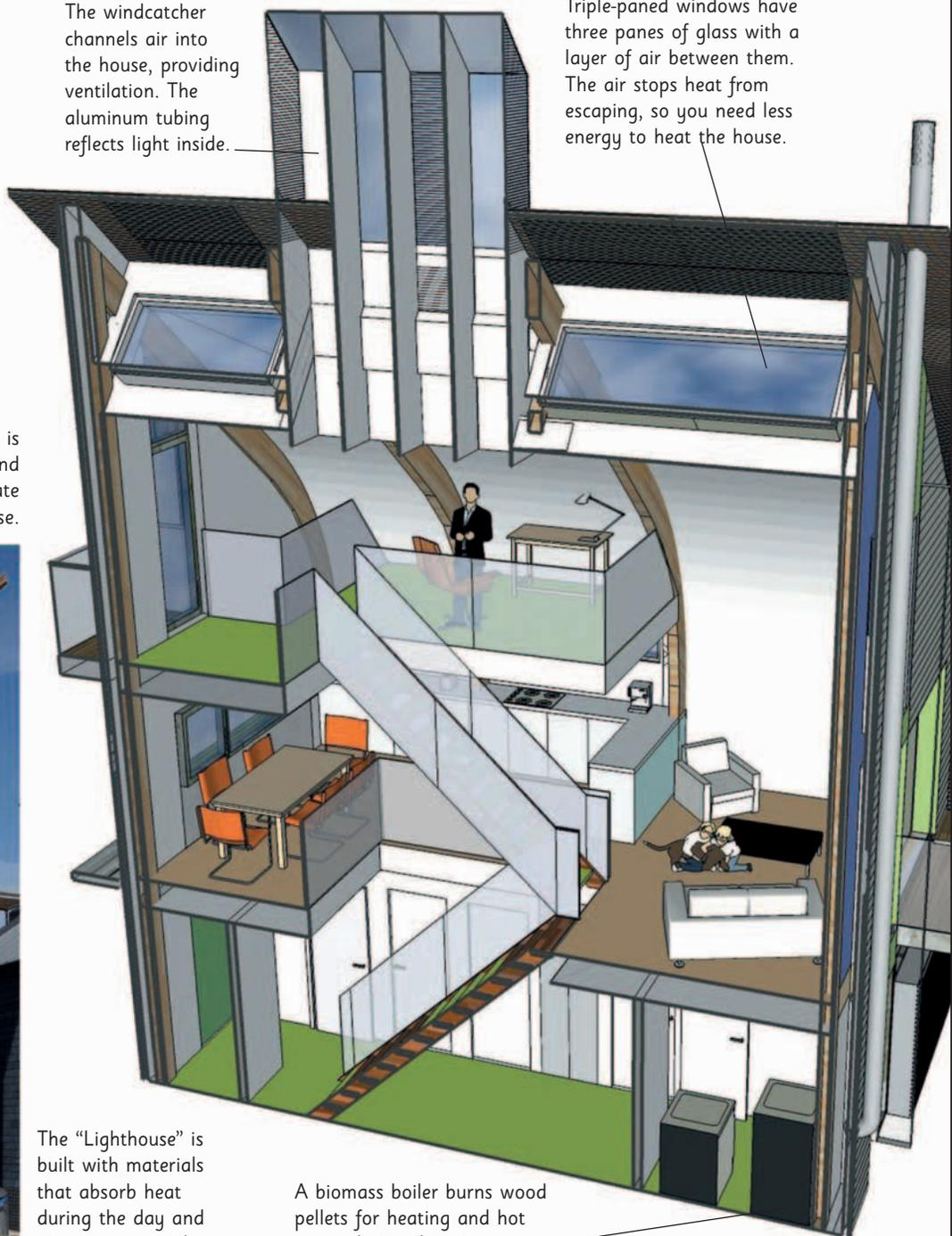
The "Lighthouse" is built with materials that absorb heat during the day and give it out at night.
