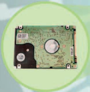
The hard drive is where all the computer's programs and data are stored permanently. Most laptops can store up to 100 gigabytes of data.
