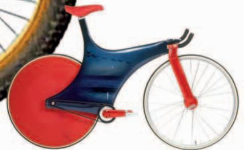
**Track-racing bikes** are designed for speed. The rider must bend low to hold the handlebars, making a streamlined shape. These bikes have no brakes!
