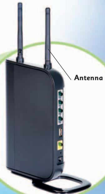
Wireless routers send and receive data through their antennae. The router then directs the data to exactly the right computer. Hubs have to try every device on the network to get the right one.
