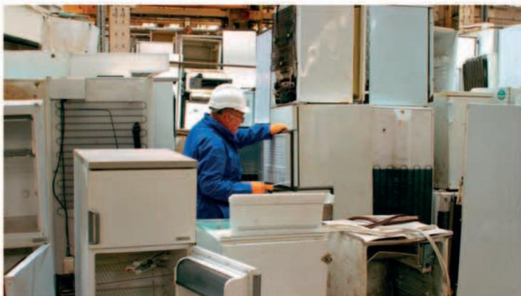
Broken fridges must be taken apart carefully so they don't release harmful gases.
