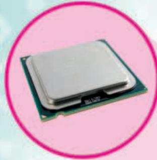
The microprocessor, or central processing unit (CPU), is the single most important chip in a computer. This electronic circuit is what makes all the programs run. It is hidden inside the computer.
