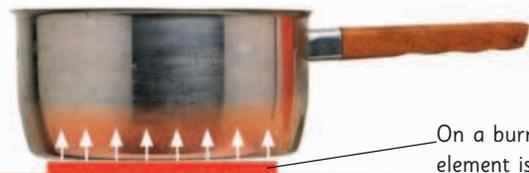
On a burner, the element is in direct contact with the saucepan, which passes the heat through to the food.
