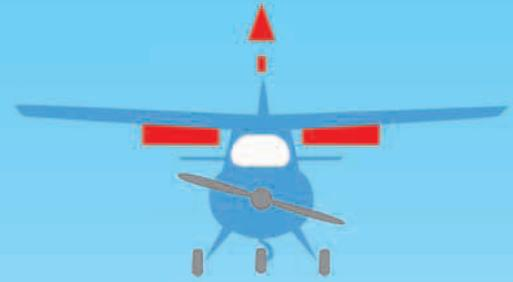
**Ailerons** on the back edge of the wings are used to "roll" the plane, to make it turn or keep it level.
