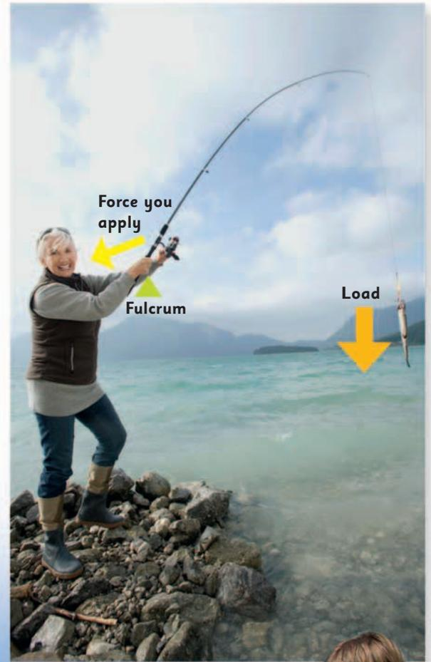
The rod also works as a class 3 lever when you haul in a fish.
