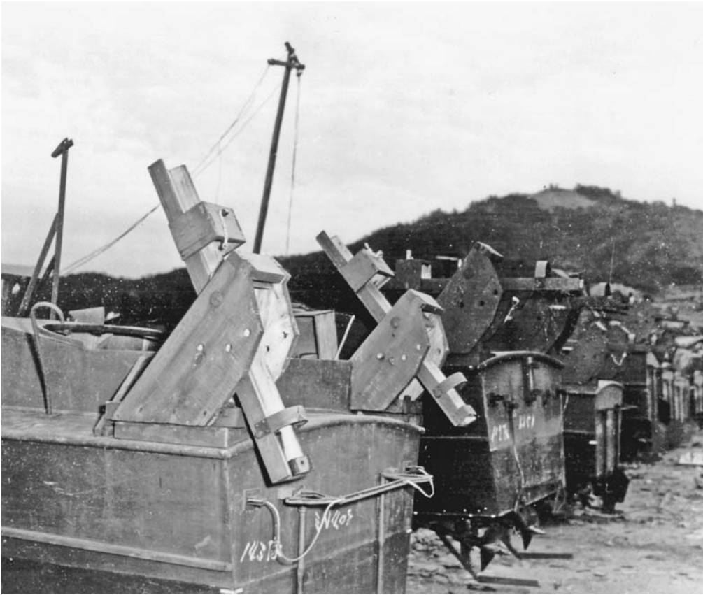
Shinyo Type 5s built near the end of the war were equipped with rocket racks on either side of the pilot. These are shown at Sasebo, Japan on 18 October 1945. Army Signal Corps Photograph.
