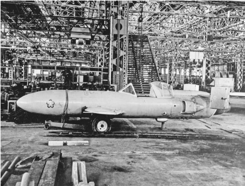
The Oka Model 22 was powered by a turbojet engine. The air intakes for the jet may be seen on the side of the fuselage. NARA 80G 193444.
