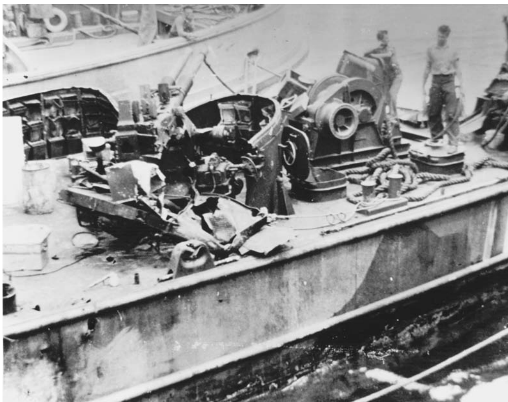
LCS(L) 116 had damage to her aft 40mm gun tub after a kamikaze attack. NARA 80G 342581.
