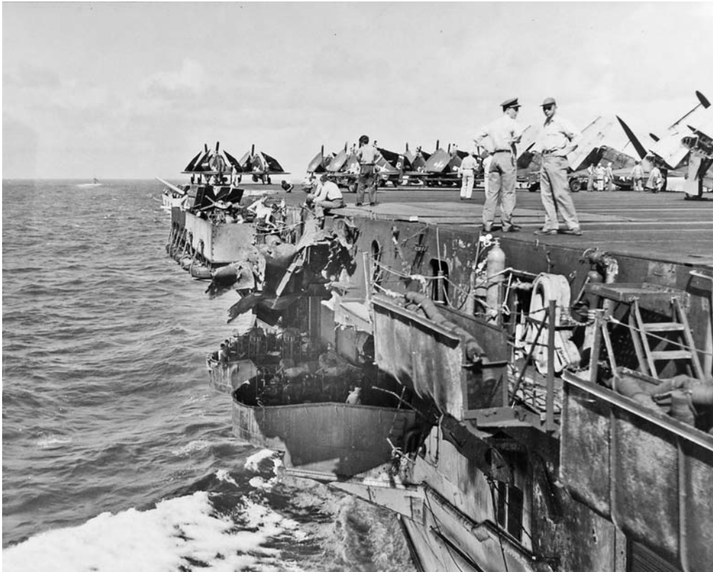
Damage to Essex CV 9 after the kamikaze attack of 25 November did not stop her and she was soon back in action. NARA 80G 270731.
