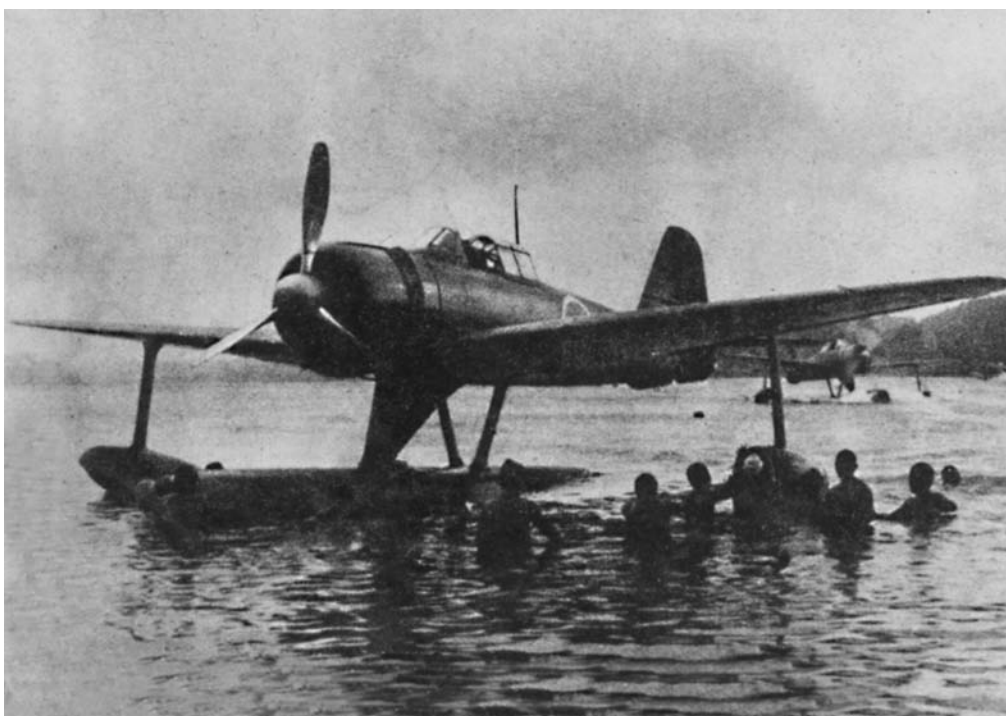
The Nakajima A6M2-N Navy Type 2 fighter seaplane carried the Allied code name Rufe. It was developed along the same lines as the Zeke. NARA 80G 169840.
