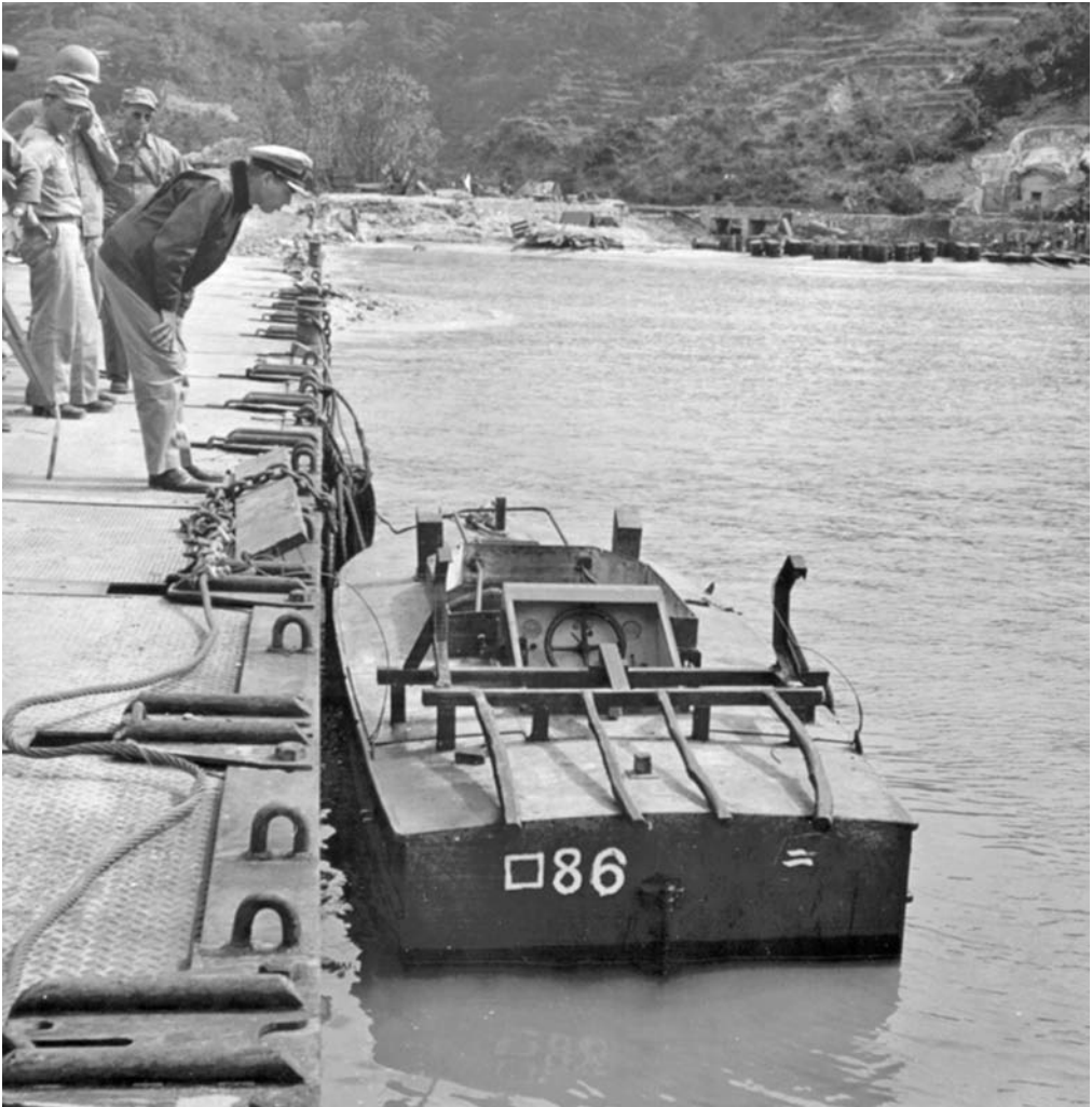
American personnel inspect a Japanese Maru-re Type 5 suicide boat at Kerama Retto on 10 April 1945. This model was used by the Japanese army. The racks aft the driver's compartment held two depth charges. Attacking the target, the pilot would swerve next to the ship and drop the depth charges which were set to go off at a shallow depth, blowing a hole in the ship. Official U.S. Navy Photograph.
