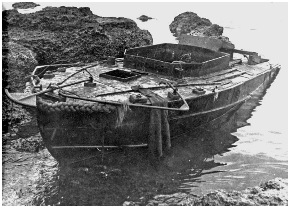
This photograph shows a Shinyo variant found in the Naha estuary on 6 July 1945. The device on the bow may have been used as a net cutter, allowing this craft to open American defenses and allow other boats through. NARA 80G 325336.
