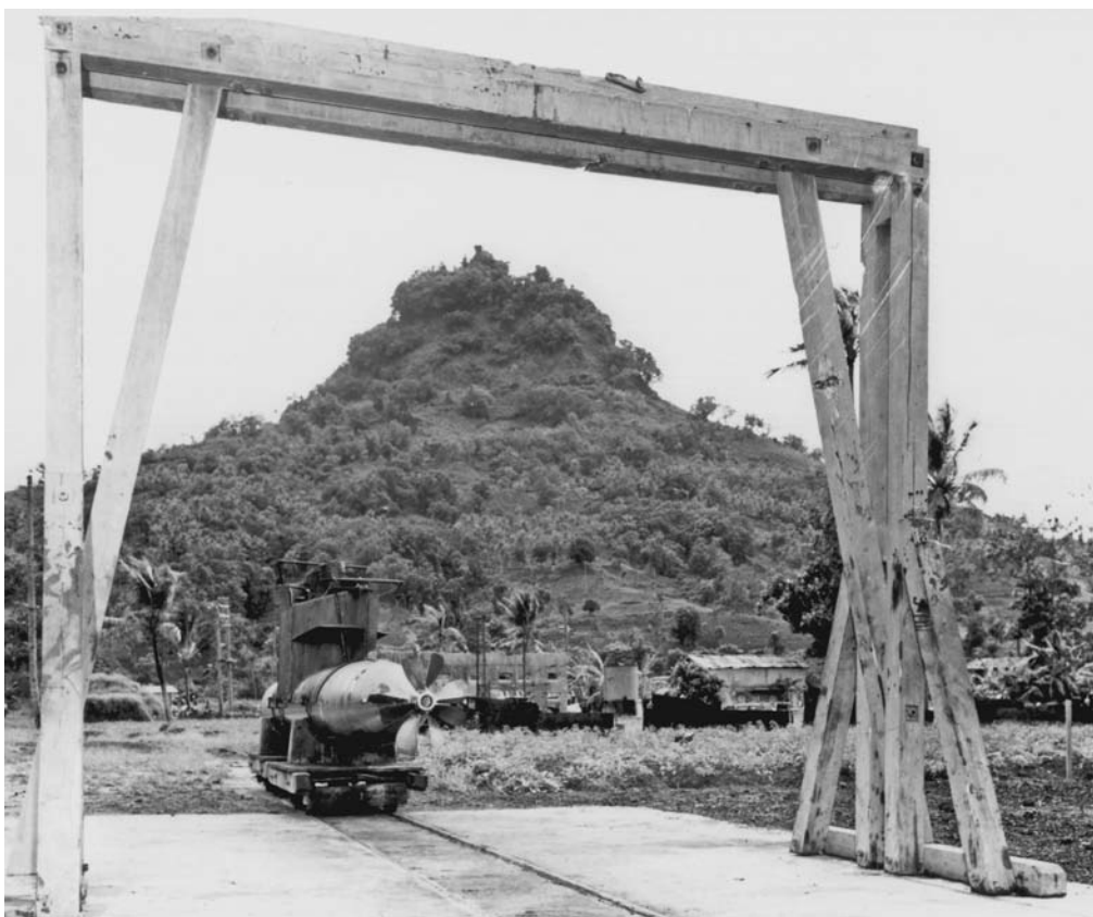
This Kaiten variant was probably designed to launch from shore to be used against amphibious assaults or anchored transports. It was captured at Truk. NARA 809G 276351.
