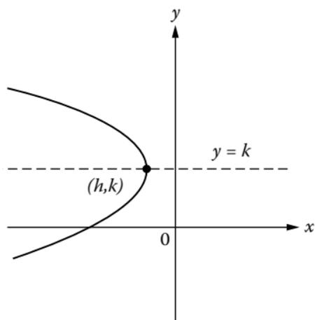
**FIGURE 4.7** Parabola with vertex at  $(h, k)$  and axis parallel to the  $x$ -axis.
