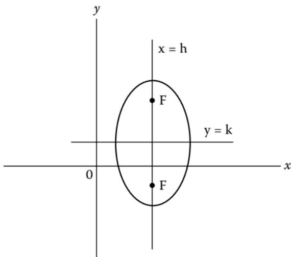
**FIGURE 4.10** Ellipse with major axis parallel to the  $y$ -axis. Each focus is a distance  $c$  from center  $(h, k)$ .
