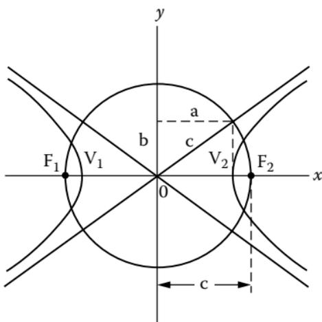
**FIGURE 4.11** Hyperbola.  $V_1, V_2$  = vertices;  $F_1, F_2$  = foci. A circle at center 0 with radius  $c$  contains the vertices and illustrates the relations among  $a, b$ , and  $c$ . Asymptotes have slopes  $b/a$  and  $-b/a$  for the orientation shown.
