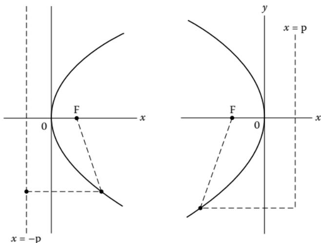
**FIGURE 4.6** Parabolas with  $x$ -axis as the axis of symmetry and vertex at the origin. Left,  $x = \frac{y^2}{4p}$ ; right,  $x = -\frac{y^2}{4p}$ .
