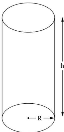
**FIGURE 1.9** Right circular cylinder.  $V = \pi R^2 h$ ;
