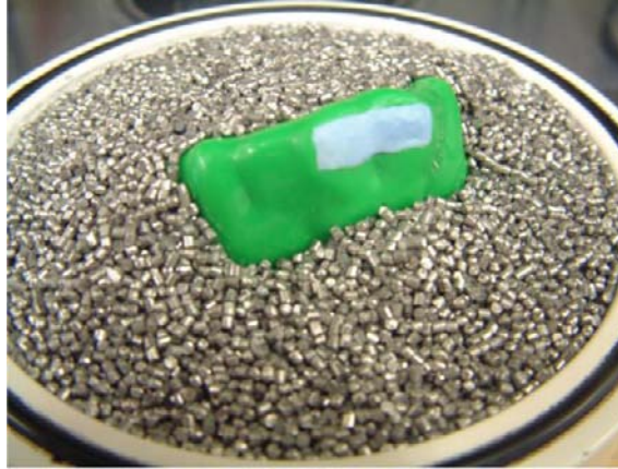
Figure 5-13. Model with first material and silicon patty is buried with granule to diminish a undercut as much as possible.
