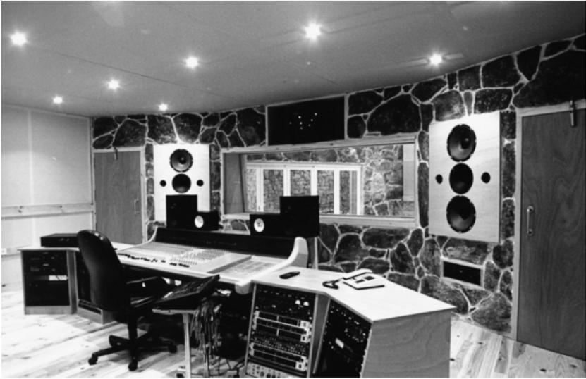
**Figure 13.10** The control room at Area Master Studios, Vigo, Spain, designed by the author, showing the vertical alignment of the drivers in the Reflexion Arts loudspeakers (1997)
