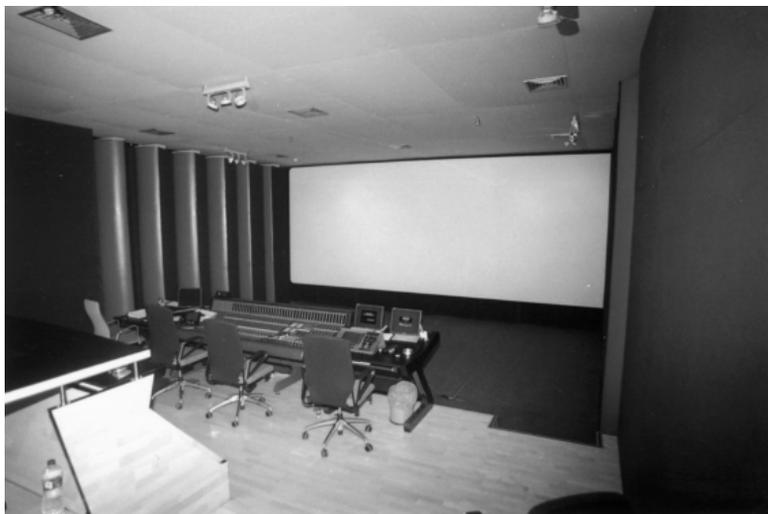
**Figure 21.9** The dubbing theatre at Soundtrack (Sala 15) Barcelona, Spain, showing the rotating acoustic control devices in the front half of the room, as outlined in Figure 7.9 (a) (ii) and (b). The front half of the room can be made more acoustically bright by rolling up the carpet and rotating the triangular panels to expose a reflective or a diffusive surface. In this mode, up to about 25 string instruments can be recorded to picture
