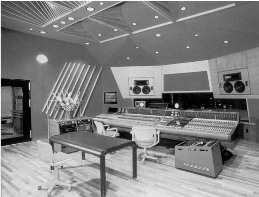
**Figure 18.4** Hitokuchi-Zaka studios, Tokyo, Japan. In this control room, designed by Shozo Kinoshita, all furniture is kept below ear height, and is positioned to avoid confusing reflections. Although the monitor loudspeakers are mounted relatively high, the size of the room ensures that the monitoring angle is kept low
