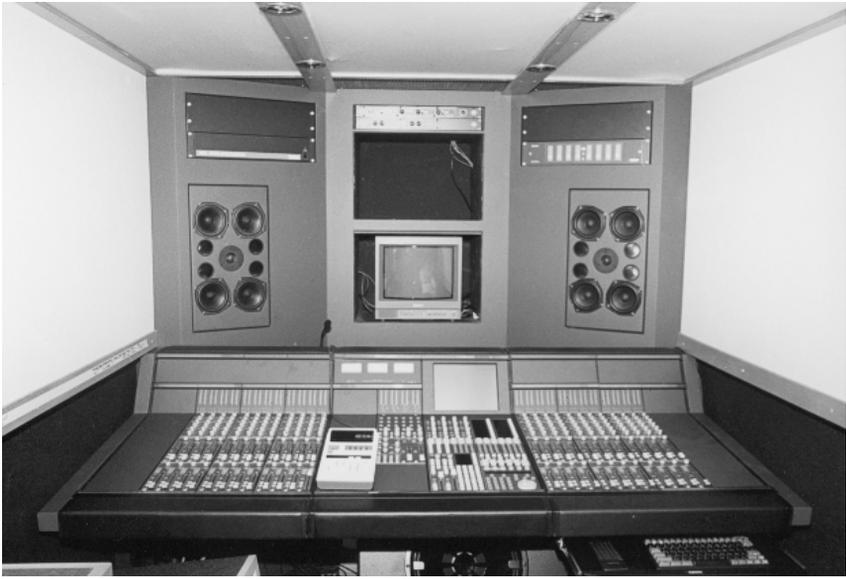
**Figure 23.17** The complete front half of the truck, with the sub-woofer just visible below the mixing console
