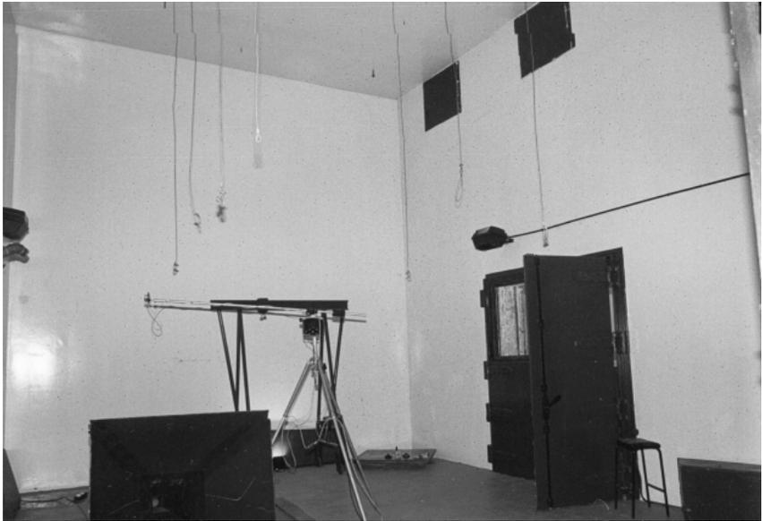
**Figure 4.1** The large reverberation chamber at the ISVR. It has a volume of  $348\text{ m}^3$  with a reverberation time of 10 s at 250 Hz, and 5 s at 2500 Hz. All surfaces are non-parallel and are made from painted concrete
