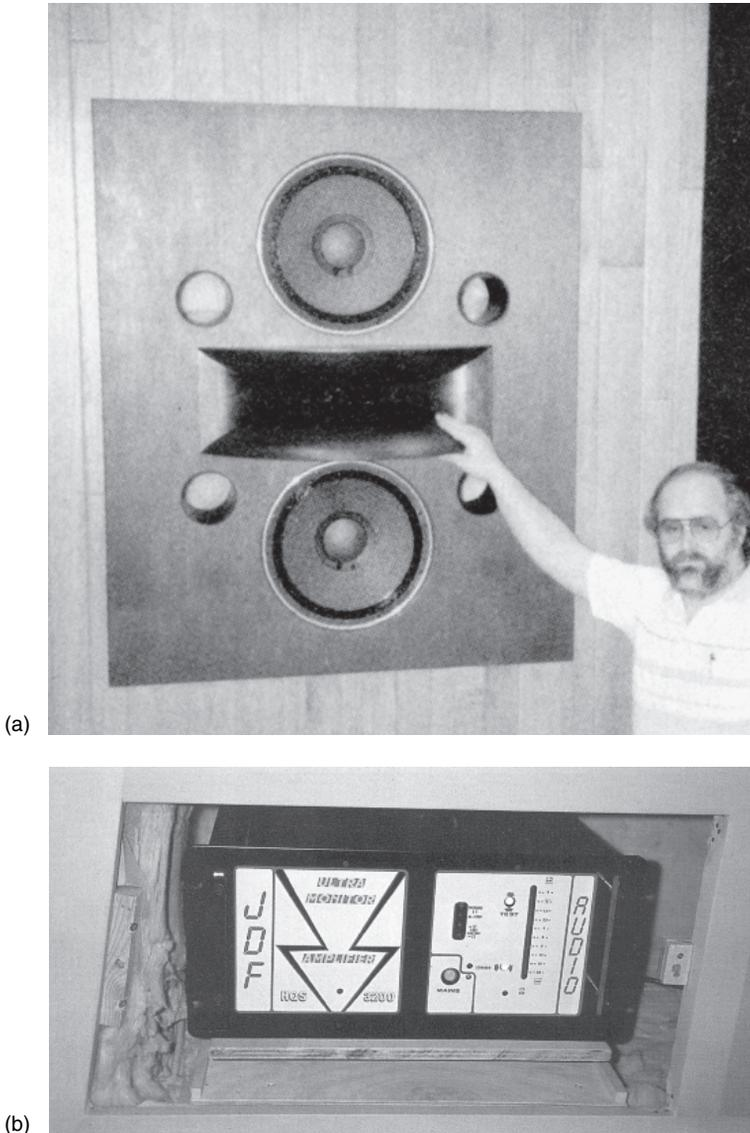
**Figure 20.1** Kinoshita '28 Hz' monitor at Masterfonics, Nashville, USA, and a typical amplifier. (a) The vertical 'D'Appolito' mounting configuration gives rise to much less response change with position when moving around in a control room. The concept allows the simplicity of a two-way system to be a practical solution for large monitors, as well as small ones. (b) A JDF amplifier, of enormous output current capacity, of a type often used with the Kinoshita monitors
