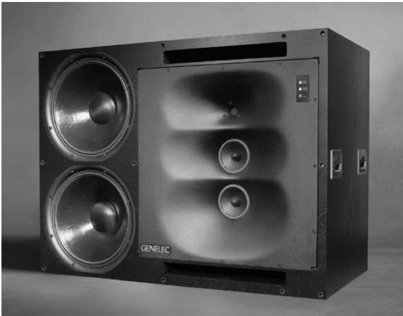
**Figure 20.11** The Genelec 1035B monitor loudspeaker. Note the 'noses' in the centre of the small mid-frequency cone loudspeakers, and the sculpted waveguide into which they are set
