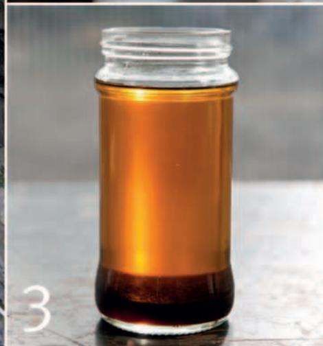
oil) with methanol. Unfortunately, if you just mix the two together, nothing will happen, so you need a catalyst. In this case, an alkali is needed and those most commonly used are sodium or potassium hydroxide.
