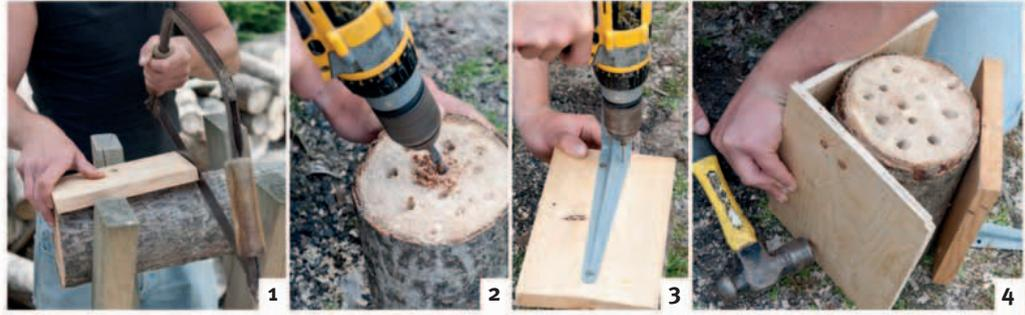
**1. Use a flat piece of wood** for the base. Cut a log section to fit the base. **2. Drill** a range of holes in one end of the log using drill bits of various sizes. Drill at a slight upward angle so that rain can't drip in. **3. Add a bracket** to the base and screw the base to the log. **4. Make a roof** with some spare wood. **5. Attach the B&B** to a south-facing wall or fence, near bee-attracting plants, and wait for the bees to move in.
