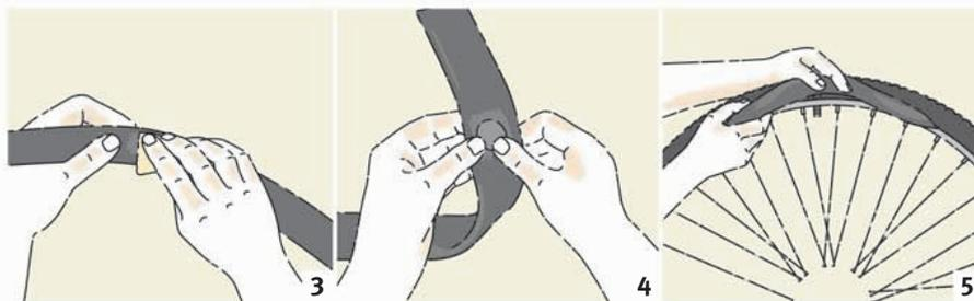
**3. Mark the hole** with chalk from your repair kit. Sand the area with sand paper, and dry the tube. **4. Apply a thin layer of glue** and wait until it starts to dry, then place a suitable patch of rubber over the puncture. Press down firmly. **5. Check the inside rim** of the tire to make sure there are no thorns or glass that will puncture it again. Fit the inner tube when it is slightly inflated.
