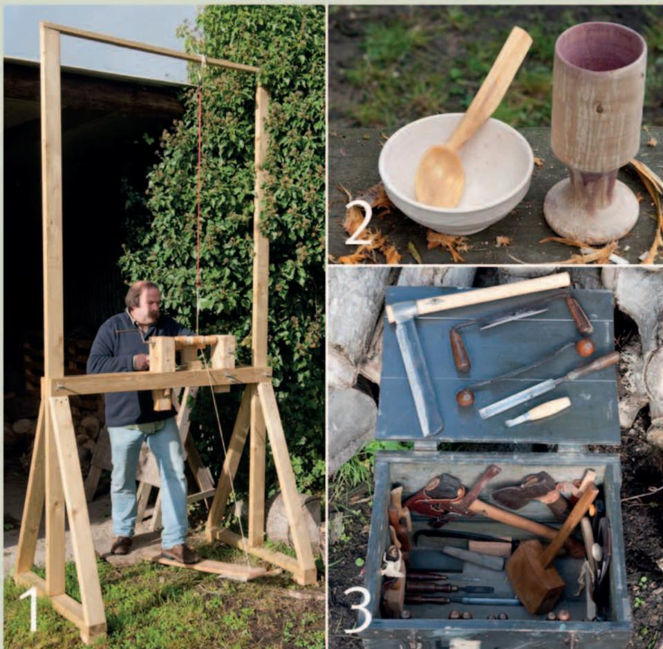
**1. A traditional pole lathe** doesn't need an electrical power supply and can be set up anywhere, even in the woods. **2. A pine bowl** and green wood goblet turned on a pole lathe, with a hand-carved cherrywood spoon. **3. Green woodworking tools**, including a froe (top left) for splitting wood and various sharp knives.
