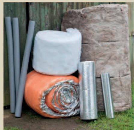
**Insulation for every situation** From left: expanded foam for pipework, recycled plastic fleece, a jacket for a hot water tank, foil reflectors for radiators, and a large roll of sheep's-wool attic insulation.
