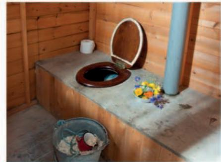
**Instead of flushing** sprinkle half a cup of sawdust down the toilet and—very important—close the lid.
