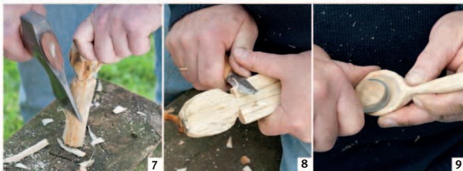
**7. Use a small ax** or a sharp knife to carve the handle. **8. Pare shavings** away from the spoon using a sharp straight knife. Be careful not to cut the spoon too thin near the neck. Try to cut over the edges of the grain, not up into them. Leave a bit of a rib on the back of the neck to give it some strength. **9. Use the hook knife** to shape the bowl. Leave to dry for a couple of days, then use it.
