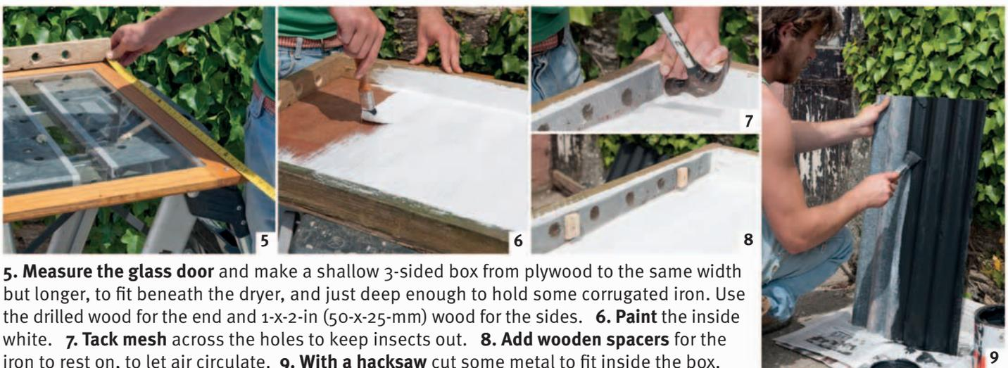
**5. Measure the glass door** and make a shallow 3-sided box from plywood to the same width but longer, to fit beneath the dryer, and just deep enough to hold some corrugated iron. Use the drilled wood for the end and 1-x-2-in (50-x-25-mm) wood for the sides. **6. Paint** the inside white. **7. Tack mesh** across the holes to keep insects out. **8. Add wooden spacers** for the iron to rest on, to let air circulate. **9. With a hacksaw** cut some metal to fit inside the box.
