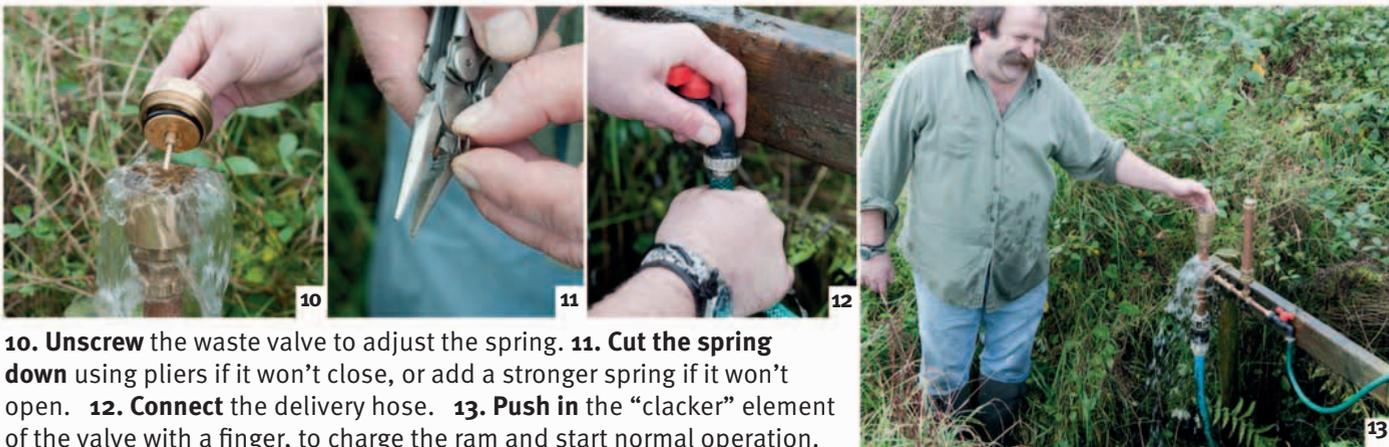
**10. Unscrew** the waste valve to adjust the spring. **11. Cut the spring down** using pliers if it won't close, or add a stronger spring if it won't open. **12. Connect** the delivery hose. **13. Push in** the "clacker" element of the valve with a finger, to charge the ram and start normal operation.
