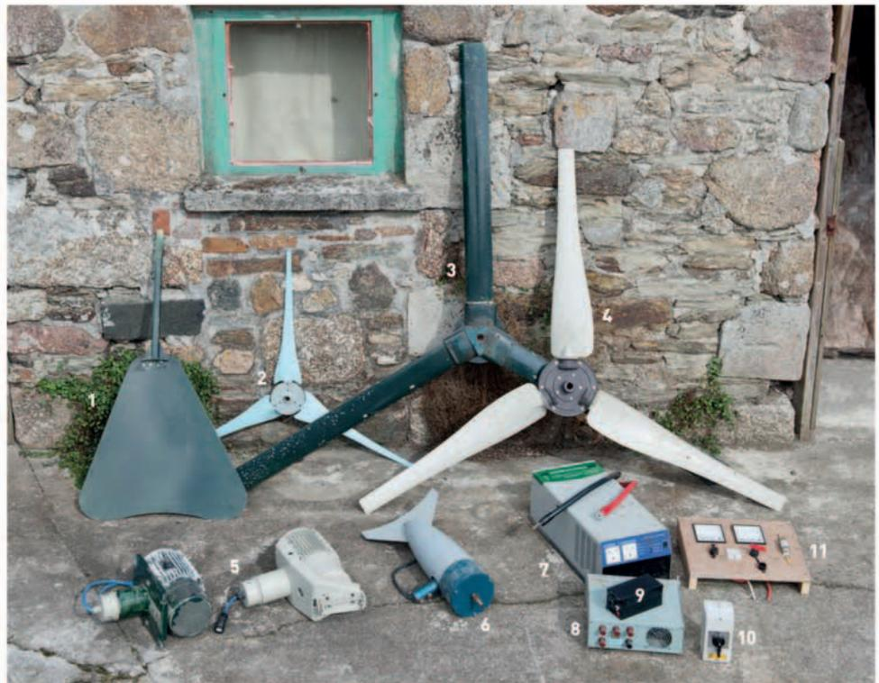
**The parts of a wind turbine** aren't numerous, but there are choices to be made for the blades, inverter, and generator. Tail furling (1), flaxing blades (2), cheap/noisy blades like planks (3), well-designed efficient blades (4), electrical generators (5), electrical generator with integrated blades (6), pure sine inverter (7), charge controller (8), cheap quasi-sine inverter (9), switch-over switch (10), and homemade monitoring capability (11).
