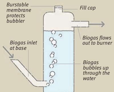
Cut a hole in the top of the cap and place a burstable membrane to limit damage.
