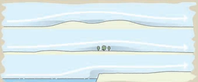
**The gray areas** above show where turbulence is created when the wind blows over hills (long areas of turbulence) and over a cliff, where the turbulence is relatively short.
