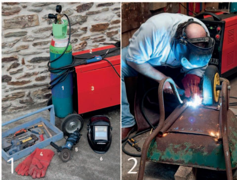
**1. The essential MIG welding kit** doesn't require a huge number of items. Above left, there is the shield gas (1), welding gun (2), welder power supply (3), heavyweight welding gloves (4), grinder (5), and welding mask (6). **2. Learn the basic skills** of welding and they can be put to use surprisingly frequently. This wheelbarrow has been a trusty friend over the years, so when its bottom fell away, a bit of tender loving care with the welder meant that all was well again.
