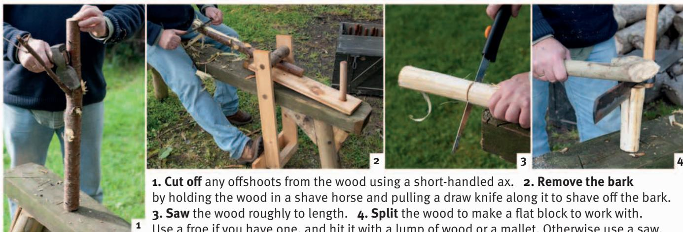
**1. Cut off** any offshoots from the wood using a short-handled ax. **2. Remove the bark** by holding the wood in a shave horse and pulling a draw knife along it to shave off the bark. **3. Saw** the wood roughly to length. **4. Split** the wood to make a flat block to work with. Use a froe if you have one, and hit it with a lump of wood or a mallet. Otherwise use a saw.
