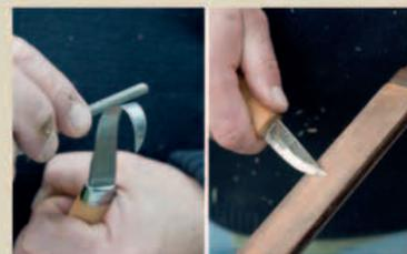
**Sharpen both cutting edges** of the hook knife with a mini steel. Draw a knife blade back and forth over a large steel to sharpen it.
