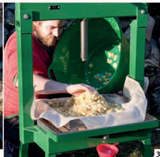
**1. Pour your apples** into the crusher, keeping your hands away from the rotating blades, having first positioned a container to catch the apples. A lower-tech means is to chop the apples in a wooden box using a spade, described below. **2. The crushed apples** will appear, as if by magic, in the container at the foot of the machine. **3. Place the mesh fabric** over the apple press base, leaving plenty of spare fabric around the edges. Spread a layer of crushed apples.
