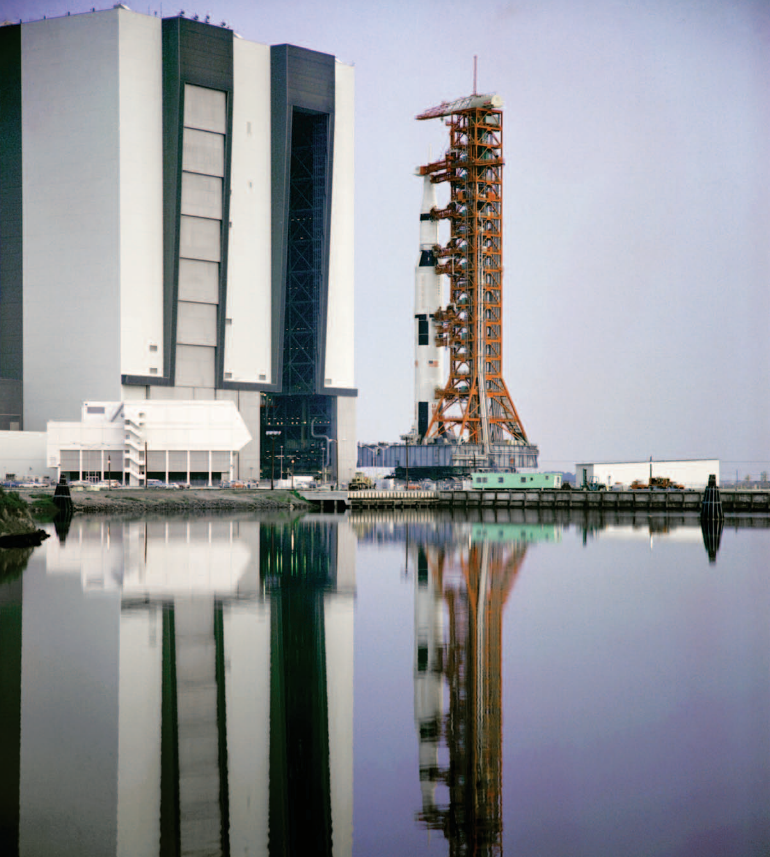
A crawler leaves the Vehicle Assembly Building carrying the Apollo 15 spacecraft and its Saturn V rocket for a 1971 mission to the Moon. It carried the first lunar rover exploration vehicle.
