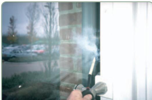
**Simple leakage test using a smoke pencil**
