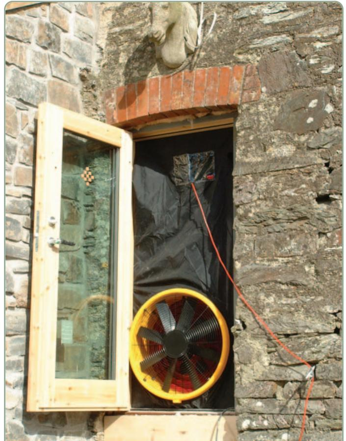
**Airtightness testing apparatus**
