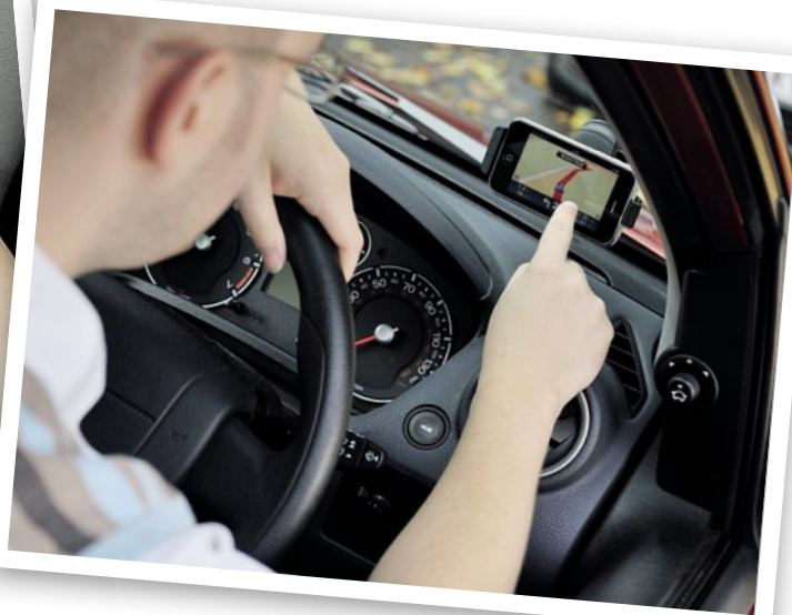
SIGNAL STRENGTH Mounting the iPhone above the dash is best for reception
