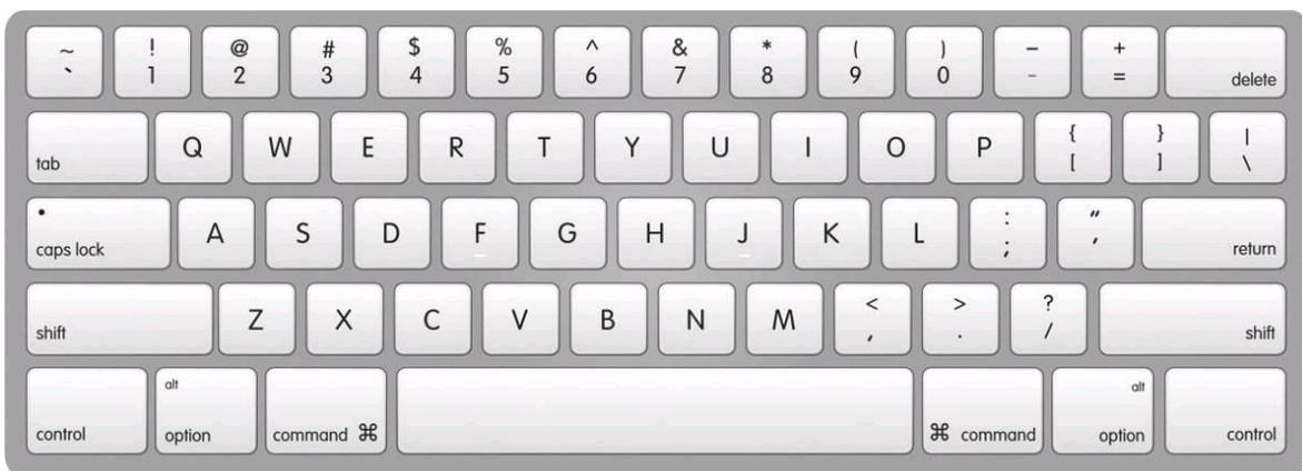
QWERTY, the argument goes, is grossly inefficient—a horrible design. There are other ways to arrange the keys on a keyboard that help the user type more quickly, accurately, and with less effort.
